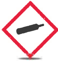
Compressed Gas Hazard
