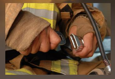
3. Attach the waist belt and adjust its tightness.
