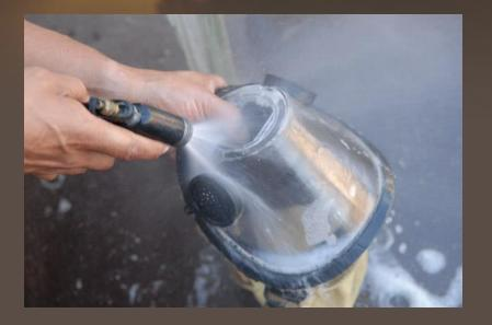
9. Completely rinse the face piece and the regulator with clean water.
