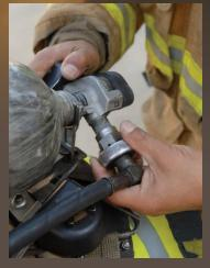
9. Connect the highpressure hose to the SCBA cylinder.
