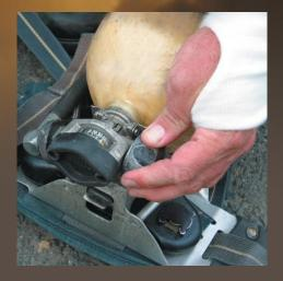
7. Shut off the air-cylinder valve.
