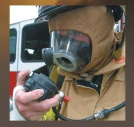
1. Remove your gloves. Remove the regulator from the face piece or disconnect the low-pressure hose. 2. Remove your helmet and pull the protective hood down around your neck.
