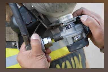
4. Disconnect the highpressure supply hose.
