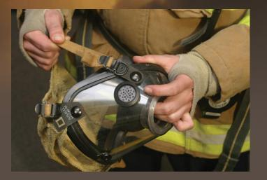
1. Fully extend the straps on the face piece.
