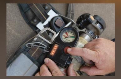
8. Open the air-cylinder valve. Compare the readings on the gauges to ensure they match.
