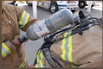
5. Release the SCBA cylinder from the backpack assembly and set it aside.
