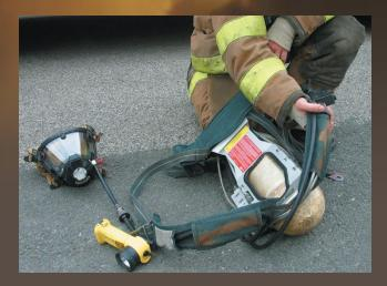
1. Open the case and lay out the SCBA. Fully open the main cylinder valve.
