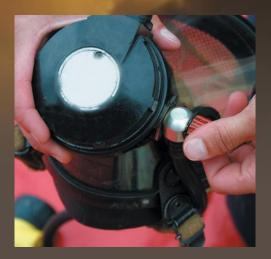
3. Open the purge valve to bleed off the pressure.
