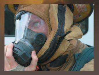
7. If necessary, connect the regulator to the face piece.
