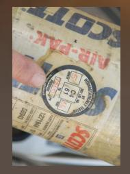
1. Remove the air cylinder from the SCBA harness and check the hydrostatic test date.
