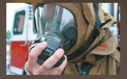
7. Replace the helmet and hood, and secure the chin strap. If necessary, connect the regulator to the face piece. Activate the air flow and PASS alarm.
