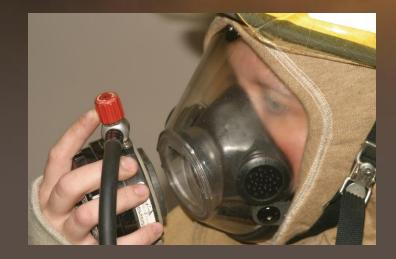
6. If necessary, connect the regulator to the face piece.Activate the air flow and PASS alarm.
