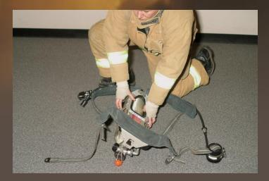
1. Open the case and lay out the SCBA with the cylinder valve away and the shoulder straps to the side.
