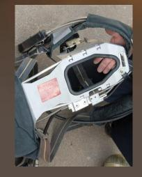
3. Inspect the SCBA shoulder straps and waist belt for damage, cuts, burns, or wear.
