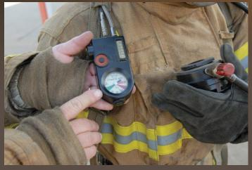
10. Open the cylinder valve and notify the fire fighter that the SCBA cylinder change is complete.
