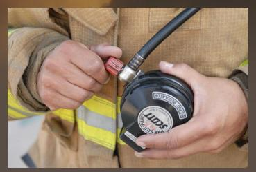
3. Open the purge valve to bleed off pressure from the high-pressure supply line.
