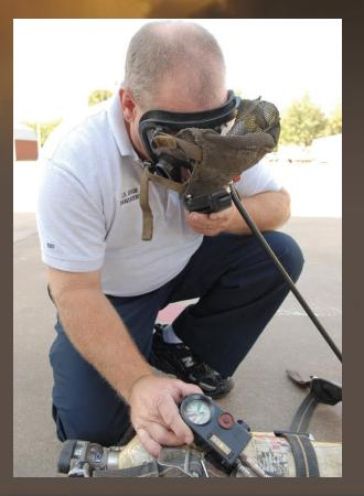
9. Attach the face piece and check the regulator for proper operation and test the PASS alarm and low-pressure alarm.
